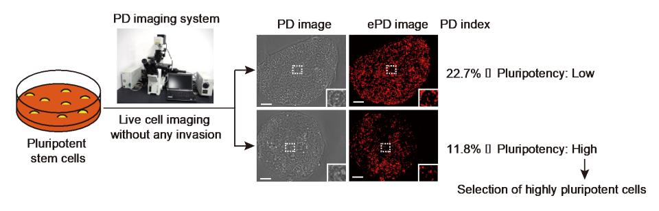
We developed an imaging system, termed Phase Distribution (PD) imaging system, which visualizes subcellular structures quantitatively in unstained and unlabeled cells. The PD image and its derived PD index reflected the mitochondrial content, enabling quantitative evaluation of the degrees of somatic cell reprogramming and PSC differentiation.
